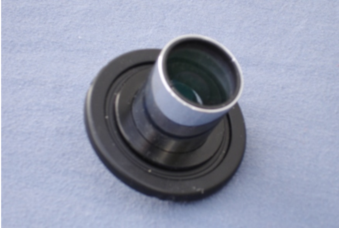
2X Barlow Celestron Ultima unscrewed and installed into a camera body cap
