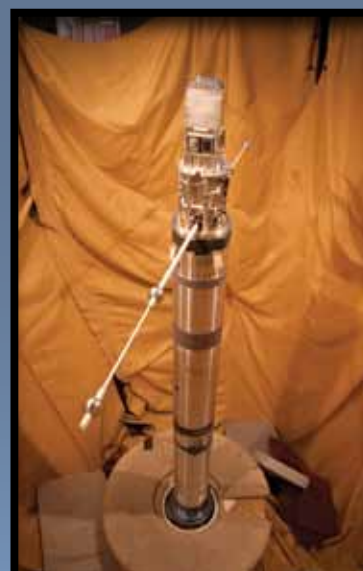
Payload boom deployment testing. Above booms folded, left booms deployed.
