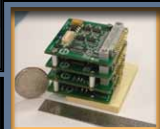
Student intern Mark Peretich and Dave Jennings installing RTAS in the Sub-TECH II payload (top). RTAS boards (above) and system layout drawing (left)
