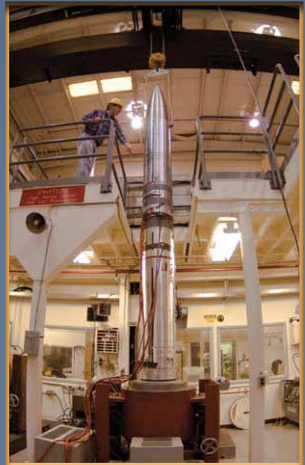
Payload on vibration table (above) and Glenn Maxfield preparing a prototype light weight mirror for vibration (left).
