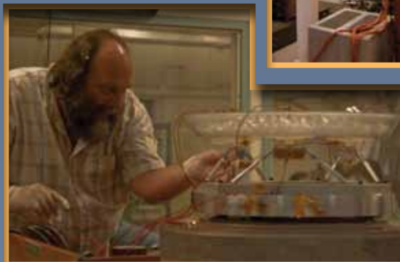
Payload on vibration table (above) and Glenn Maxfield preparing a prototype light weight mirror for vibration (left).
