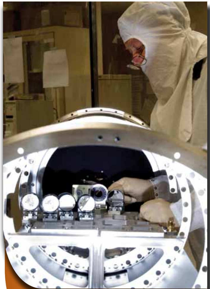
Figure 1: Marshall scientist Ed West assembles the optical system of the Solar Ultraviolet Magnetograph Investigation telescope.
