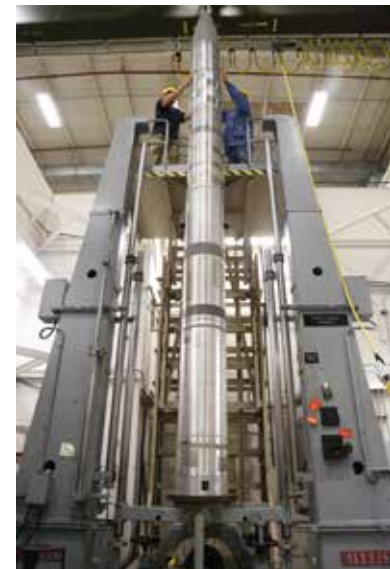
Payload being prepared for balancing.
