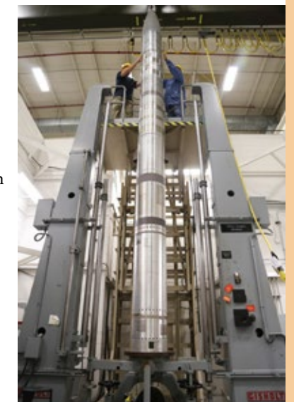
Payload being prepared for balancing. Photo by: Berit Bland/NSROC
