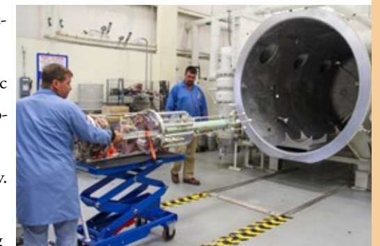
Payload ready to enter the thermal-vacuum chamber. Photo by: Berit Bland/NSROC
