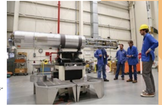
Payload placed on mass properties measurement table. Photo by: Berit Bland/NSROC
