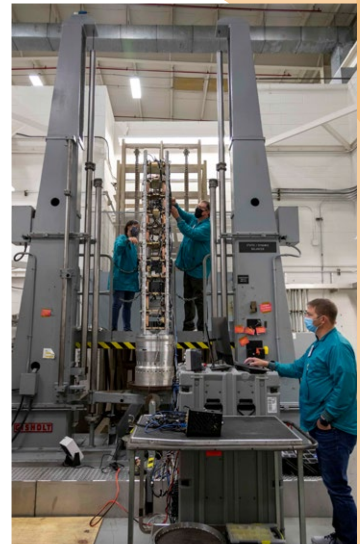
HOTShot payload during integration at Wallops. Photo by: Berit Bland/NSROC
