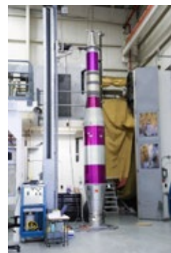
Bend testing of payload. Photo by: Berit Bland/NSROC
