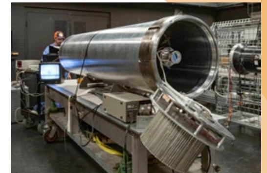
Open shutter door with instrument visible during testing at Wallops. Photo by: Berit Bland/NSROC
