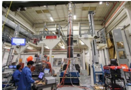
Payload on vibration table. Photo by: Berit Bland/NSROC
