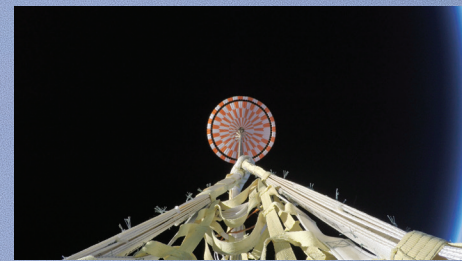
Parachute inflation imaged during flight.
