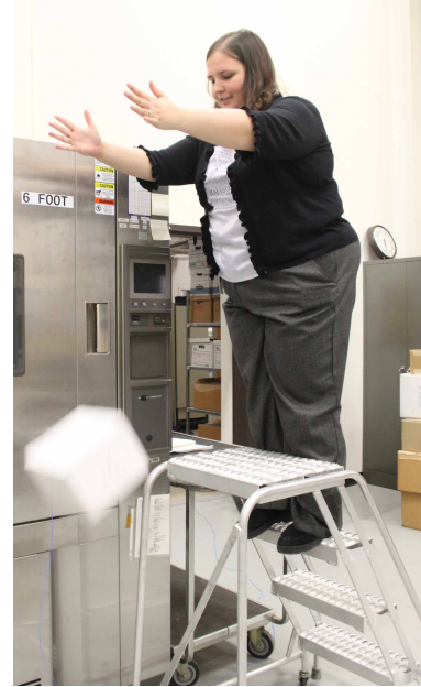
Lindsey drop testing FTS batteries.
