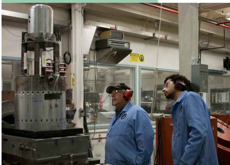
Tom and Paul vibration testing a new deployment mechanism for the Daytime Dynamo missions.
