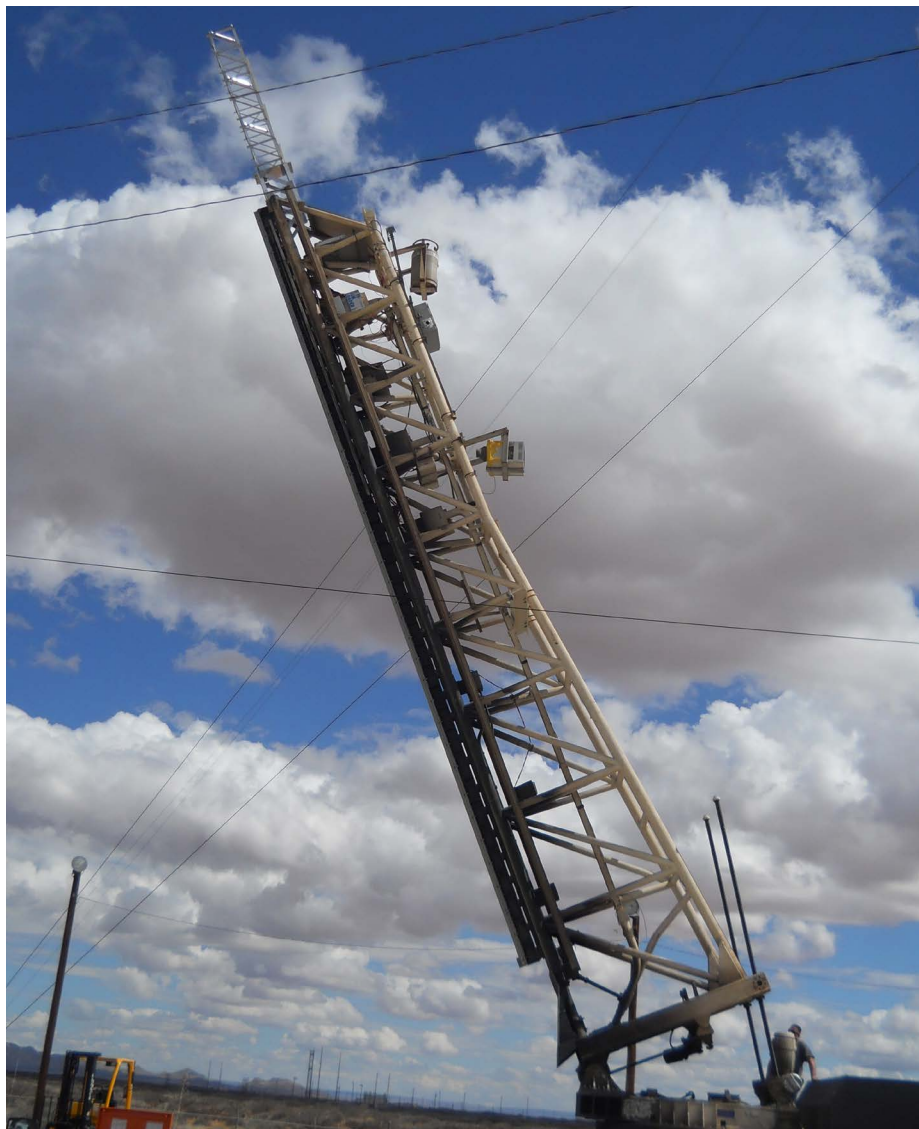
Launcher operational checks to verify the general operation of the launcher and its limit switches.
