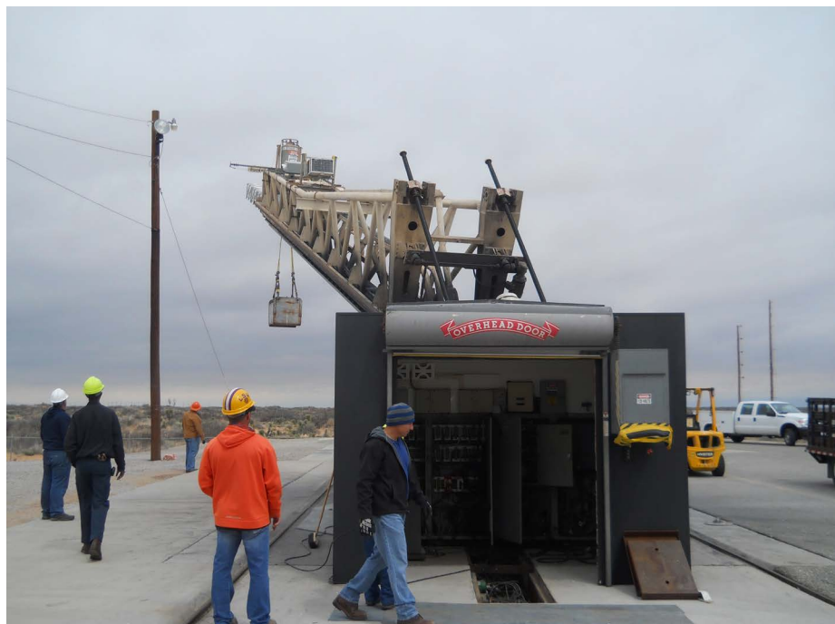
Launcher boom load test.
