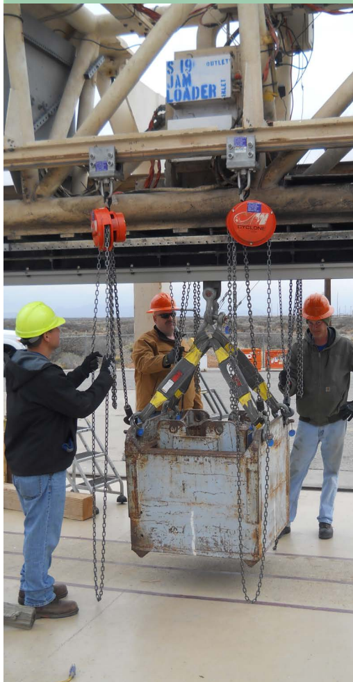
Launch rail load test.
