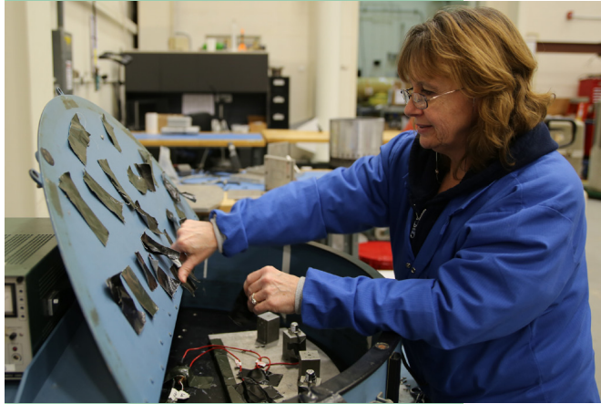
Pat testing accelerometers in the centrifuge.
