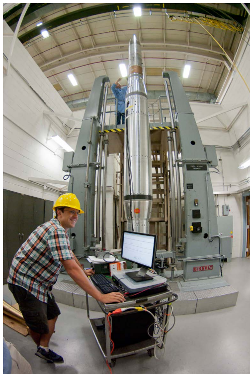
FORTIS on the spin balance table in the Testing and Evaluation lab.
