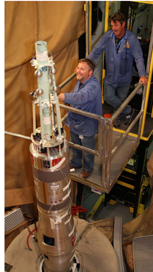
Stowing booms on the CARE payload after successful deployment testing.
