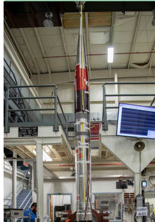
RockSat-X on the vibration table.
