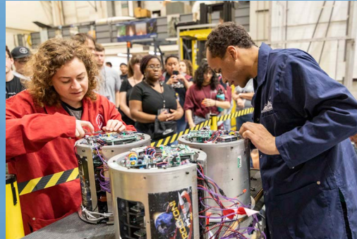
Preparing RockOn! canisters for integration.
