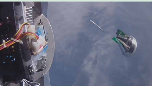
Image of REX SAT-X deploying captured by onboard HD video camera.
