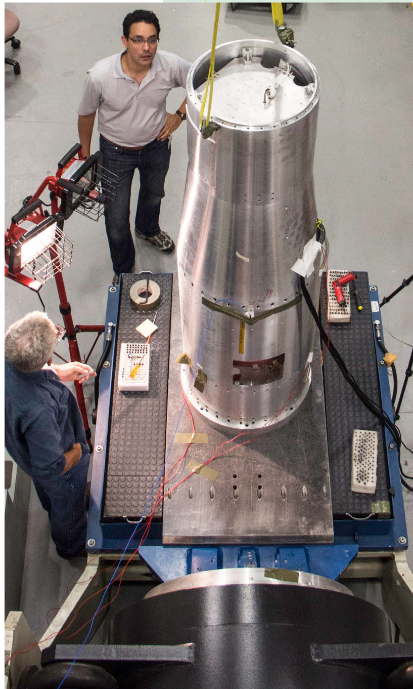
The Adiabatic Demagnetization Refrigerator (ADR) for the Micro-X mission at Wallops for vibration testing.
