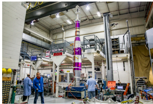
ASPIRE on the vibration table.
