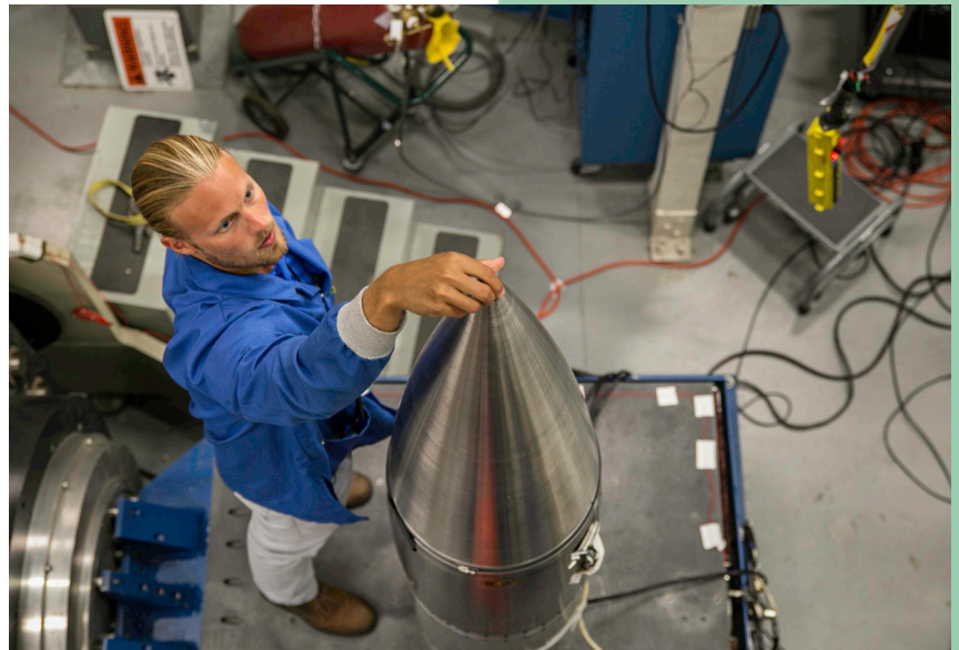
N-FORSe vibration testing.
