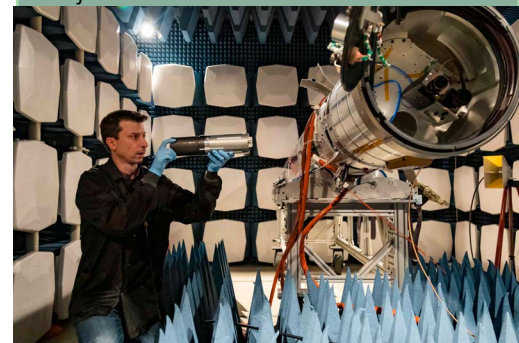
Sub-payload testing in the EMI chamber.
