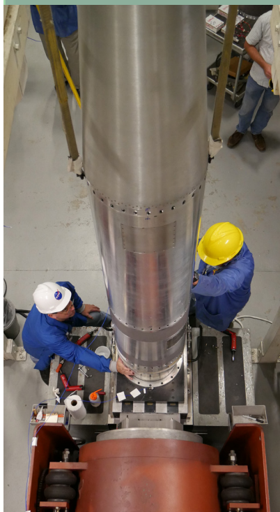
Azeem payload on the vibration table.
