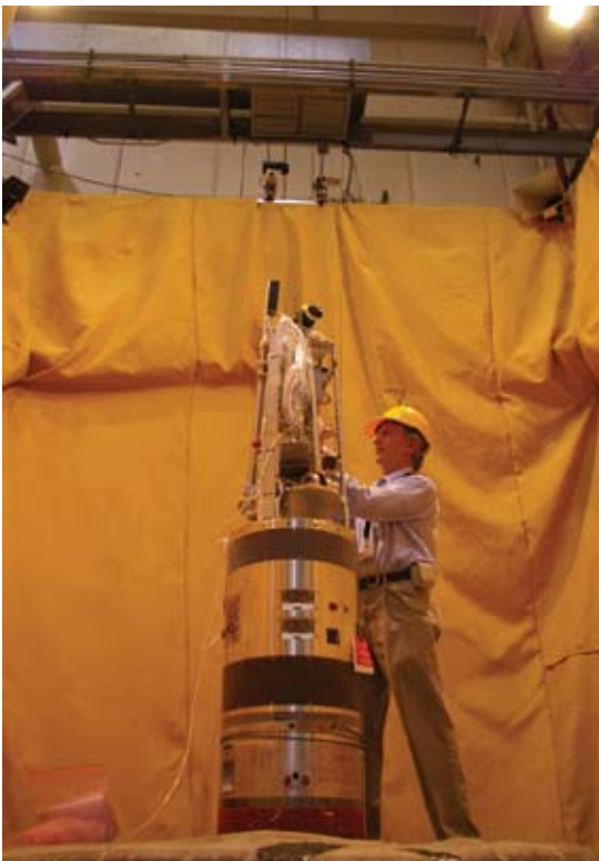
SCIFER-2 in the spin/deployment facility at Wallops.
