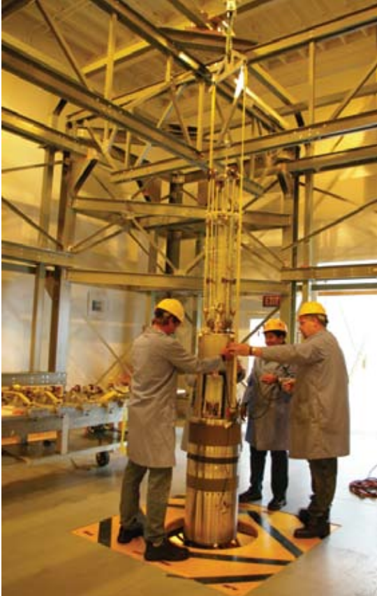
TRICE payload in the magnetic calibration facility at Wallops.
