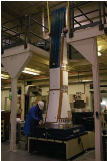
HyBolt on the vibration table at Wallops.
