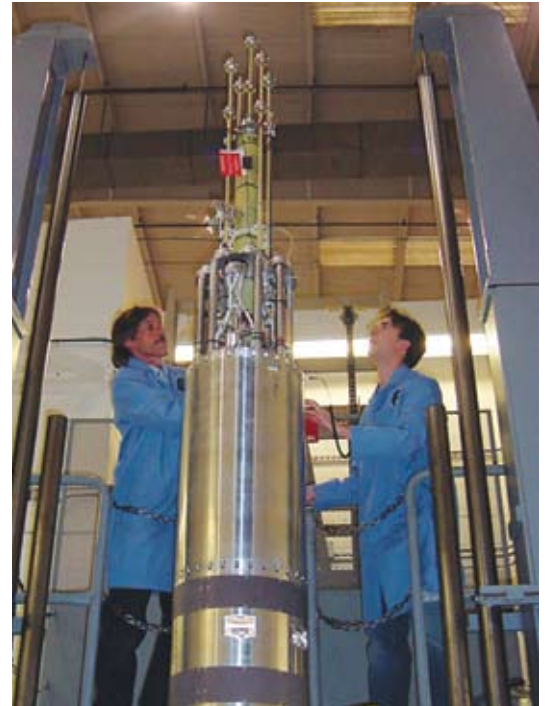
CHARM payload on the spin/balance table.
