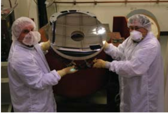
Ultra Light Weight mirror post vibration at Wallops
