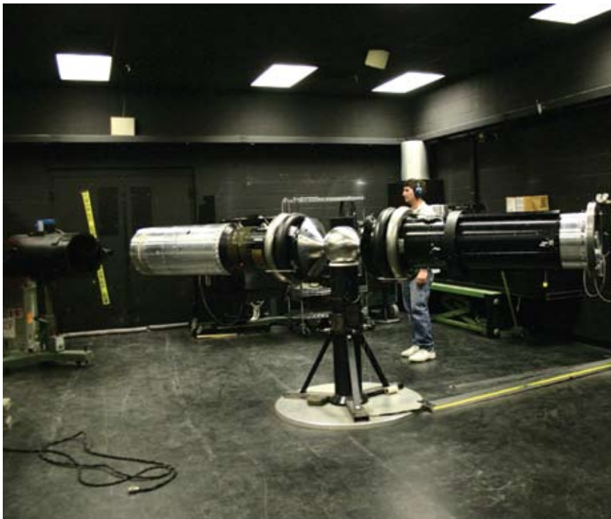
The Celestial Attitude Control System airbearing test.
