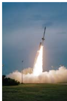
Terrier-ASAS motor test round, June 2005
