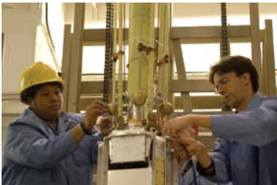
Payload in spin/balancing facility at Wallops
