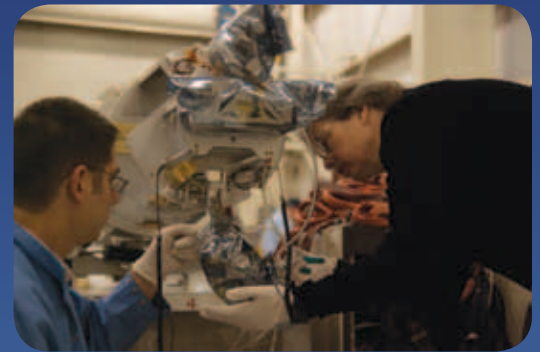
Brian Creighton and Dr. Kristina Lynch (PI) testing boom release mechanism.
