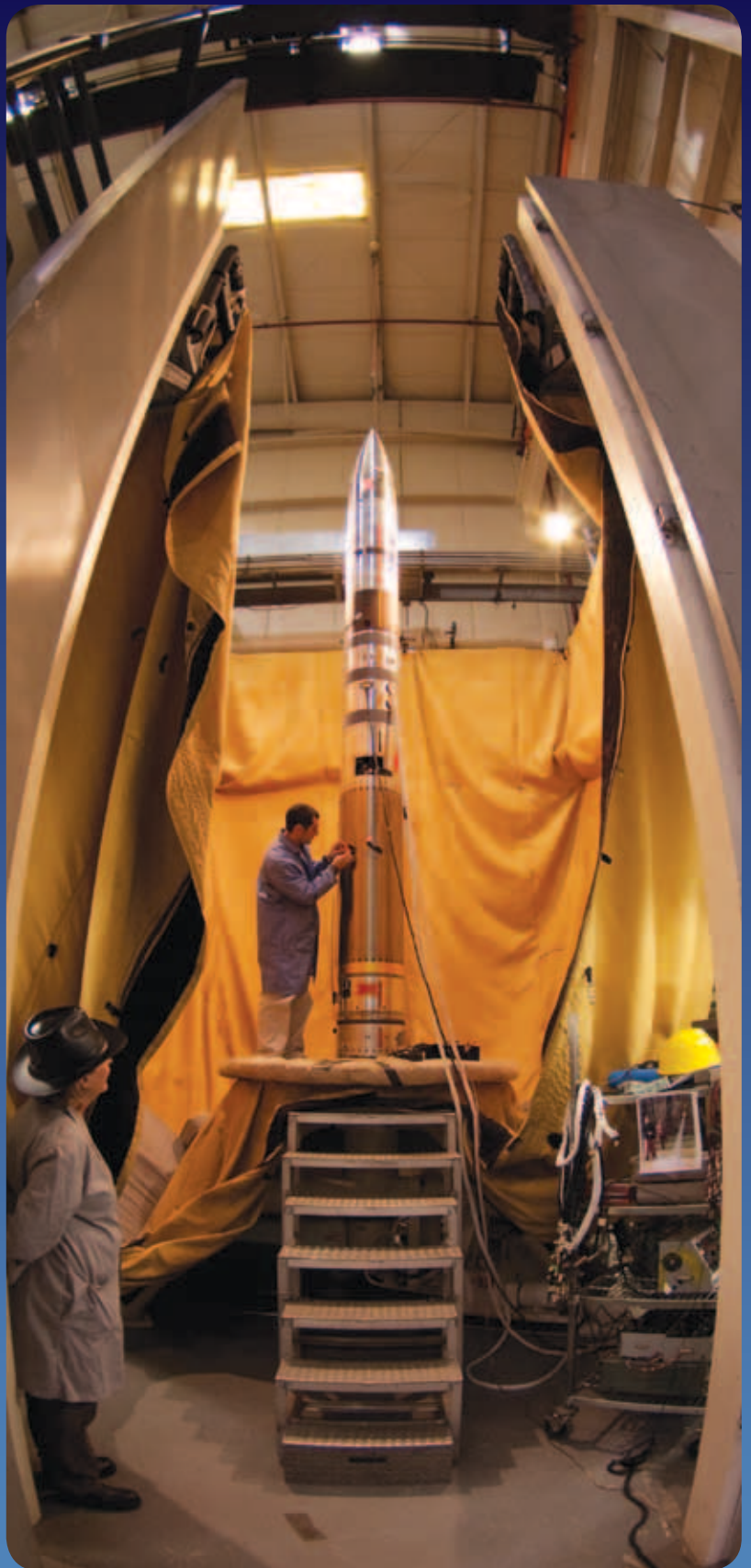
36.226 UG payload being prepared for deployment testing.
