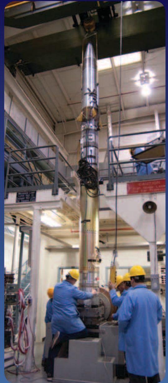
Payload being prepared for vibration testing in the T&E lab.
