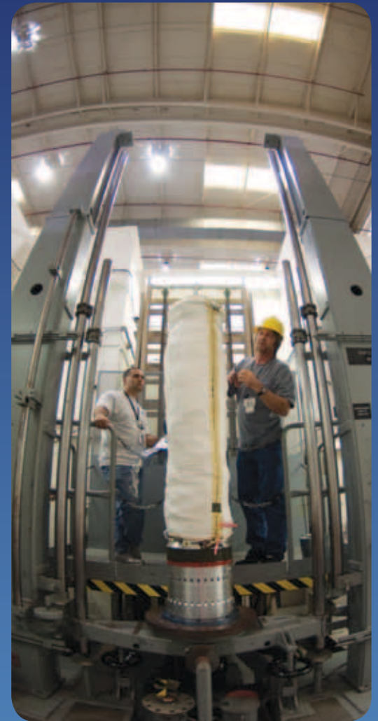
Stowed IRVE on the spin/balance table at Wallops.
