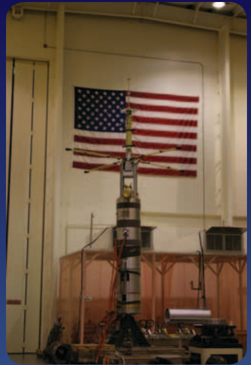
Boom deployment testing.
