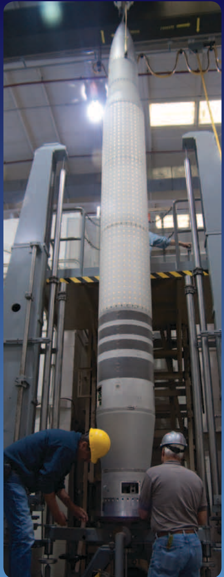
MARTI payload on balancing table.
