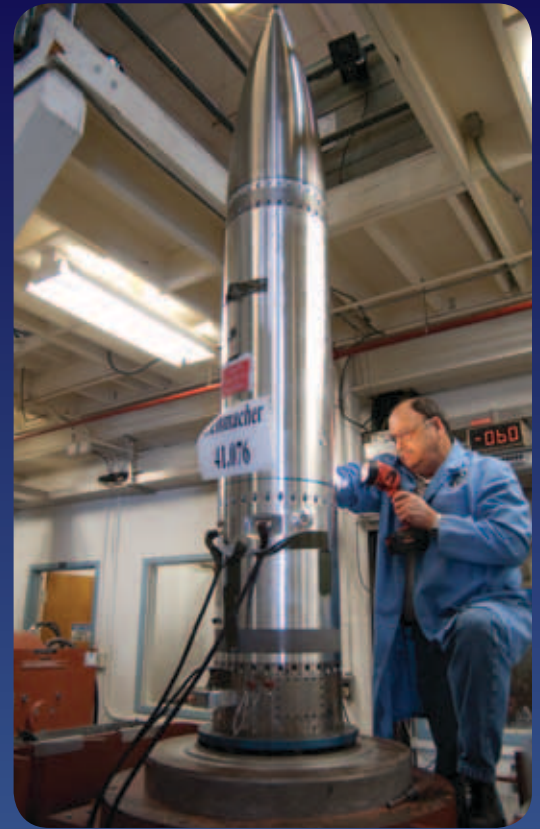
41.076 on the vibration table in the Testing and Evaluation lab at Wallops.
