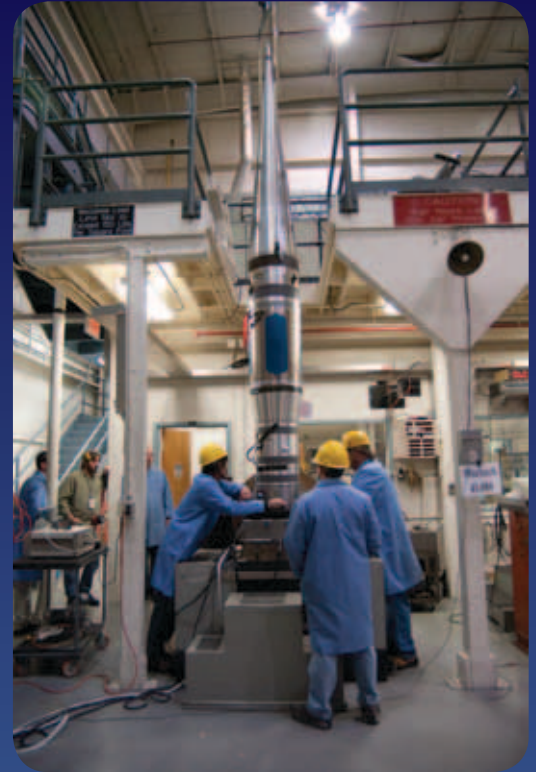
Payload being prepared for vibration testing in the T&E lab.
