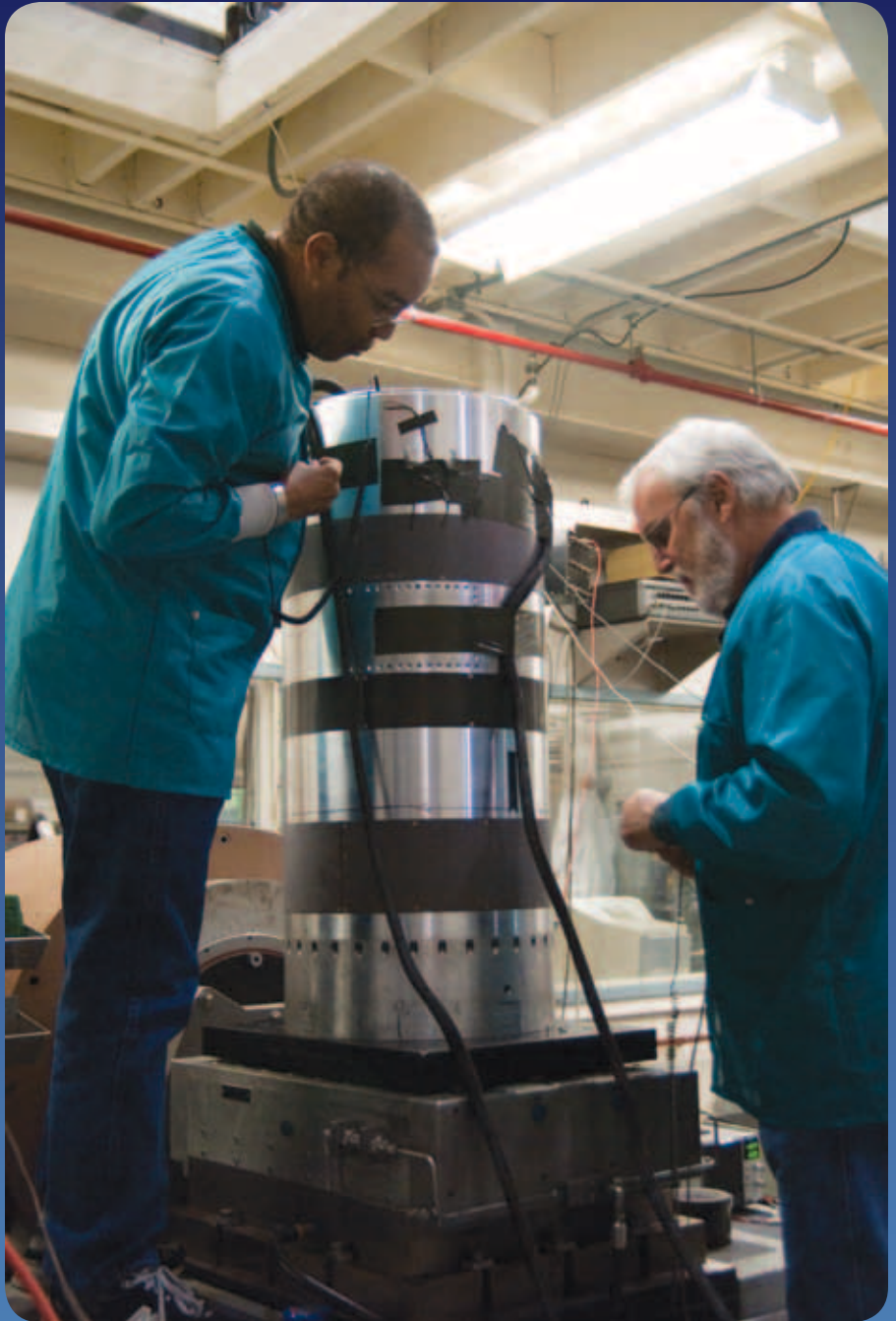
Greg Waters and Bob Ray preparing the AFSS for vibration testing.
