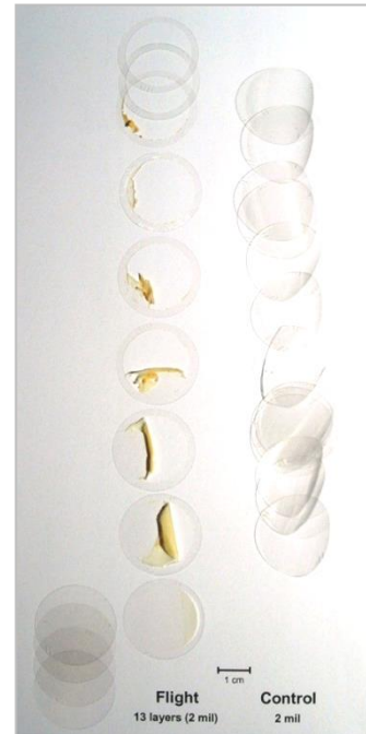
Post-flight photograph of individual sample layers. Layers were separated for weighing. (Mass loss Situation 2)
