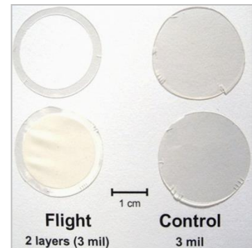
Post-flight photograph of individual sample layers. Layers were separated for weighing. (Mass loss Situation 2)
