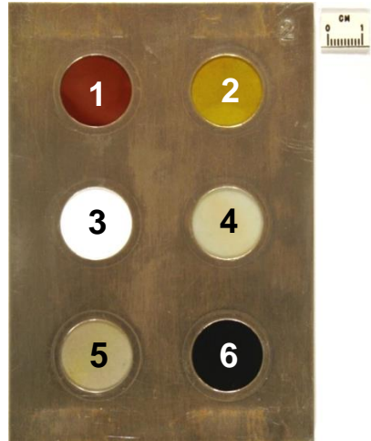
Figure 45—Sample Holder with Six Polymer Samples
