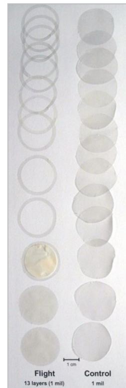
Post-flight photograph of individual sample layers. Layers were separated for weighing. (Mass loss Situation 2)
