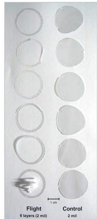
Post-flight photograph of individual sample layers. Layers were separated for weighing. (Mass loss Situation 2)
