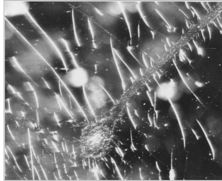
(b) Post-Flight with Mud-Tile Cracking Observed
