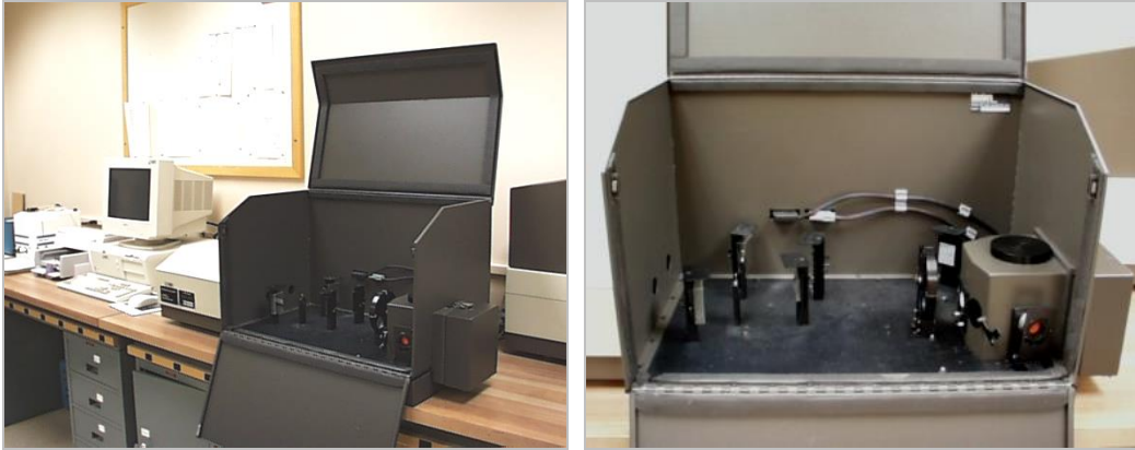
Figure 58—Perkin Elmer Lambda 19 Spectrophotometer with Closeup of Integrating Sphere
