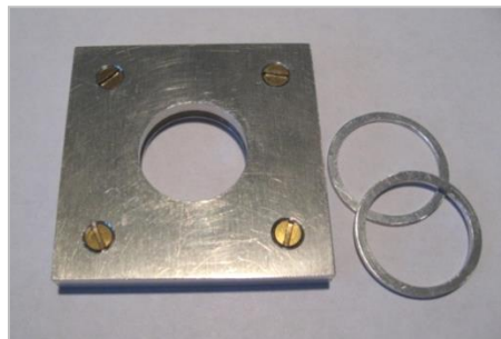
Figure 57—Sample Holder for Optical and Thermal Measurements
