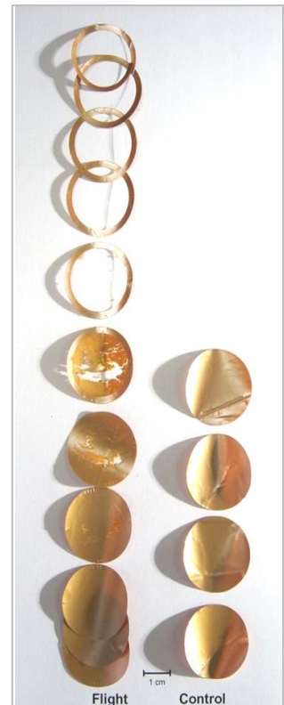
Post-flight photograph of individual sample layers (11 flight; 4 control). Layers were separated for weighing postflight. (Mass loss Situation 2)
