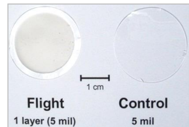
Post-flight photograph of stacked sample layers. Sample layers could not be separated for weighing. (Mass loss Situation 1)
