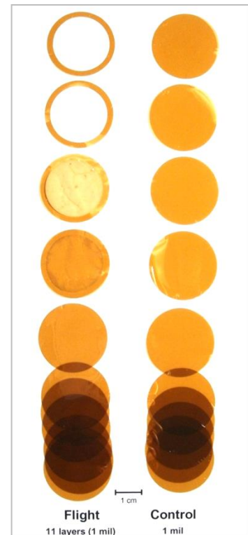
Post-flight photograph of individual sample layers (11 flight; 10 control). Layers were separated for weighing. (Mass loss Situation 1)
