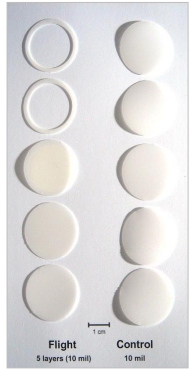
Post-flight photograph of individual sample layers. Layers were separated for weighing. (Mass loss Situation 1)
