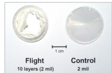
Post-flight photograph of stacked sample layers. Layers could not be separated for weighing post flight. (Mass loss Situation 3)
