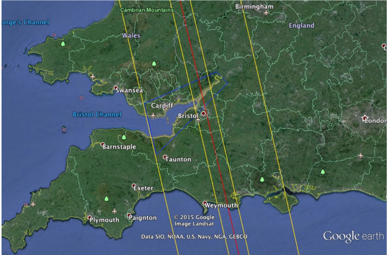
Figure 75. River Severn study site (blue polygon) covering the area from the seaward limit of the SWOT fast sampling orbit swath upstream to where the channel width decreases below ~100m.
