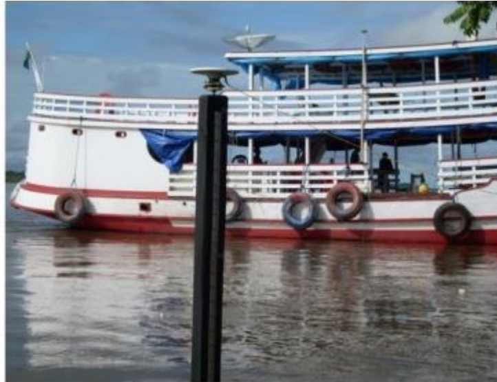
Figure 58. Leveling of a gauge by direct observation with a GPS system on top of a gauge (foreground), and survey of the river height and slope with a GPS system installed on the roof of the boat (background).
