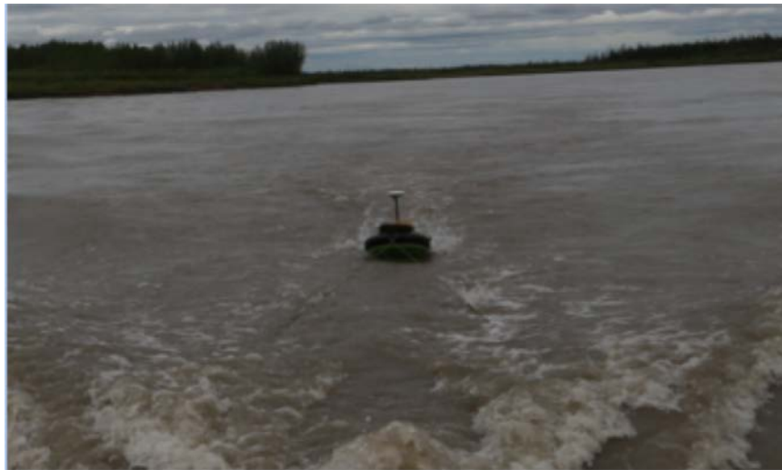
Figure 22. The Sontek hydroboard system that will also be used to produce precision GPS measurements of water surface elevation.
