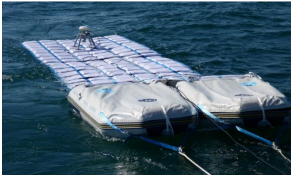
Figure 21. The CalNaGeo instrument used to produce the highest precision water surface elevations from GNSS measurements.
