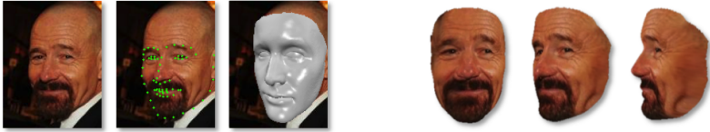
Fig. 2: Adding pose variations by synthesizing novel viewpoints. Left: Original image, detected landmarks, and 3D pose estimation. Right: rendered novel views.
