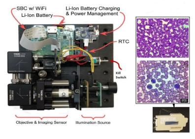
At left, the scope's single board computer features rechargeable operation and built-in WiFi. On bottom-right, a self-contained slide staining device (by the same inventors) allows quick viewing of biological cells such as this blood smear.
