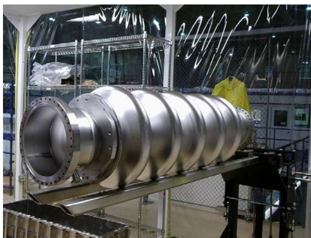
Figure 3-7. The ERL 5-cell accelerating cavity.
