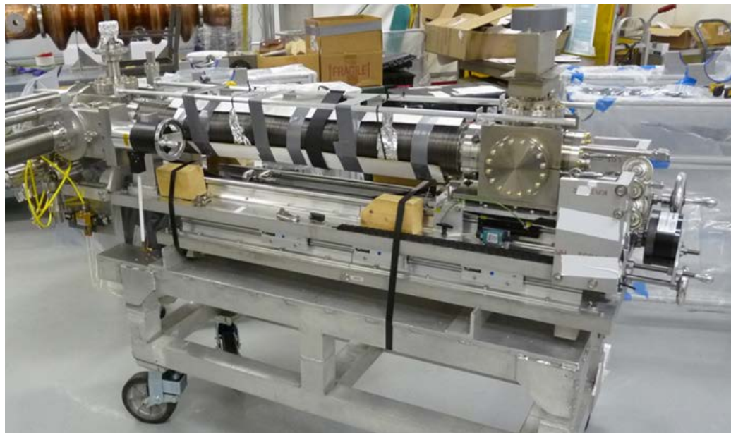
Figure 3-3. The UHV transport cart element of the load lock system.
