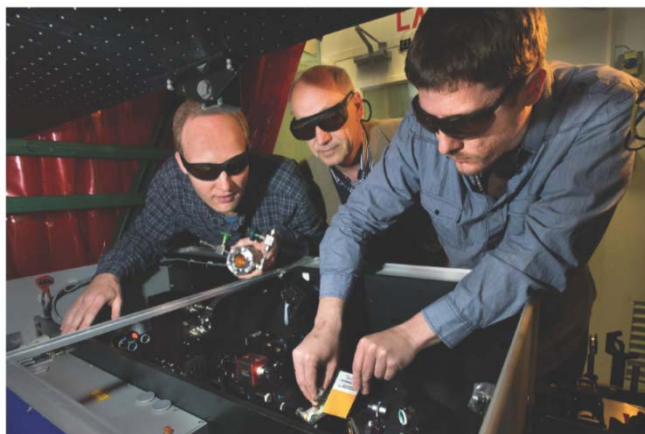
Figure 2-13. Compact solid state femtosecond OPA manufactured by Quantronix Co. (left) opened for alignment by the ATF laser operators (right).
