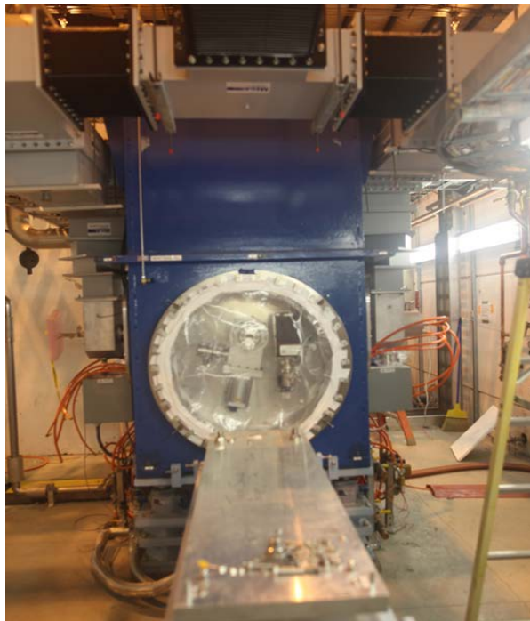
Figure 3-6. The cryomodule of the SRF gun seen from the cathode insertion port side.
