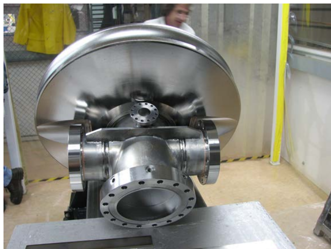
Figure 3-5. SRF photocathode electron gun, 2 MeV 300 mA at 704 MHz. The beam port faces front, the twin fundamental power couplers to the right and left, the pick-up probe facing upwards.
