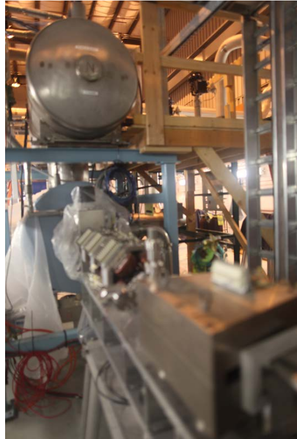
Figure 3-8. The linac cryomodule of the ERL, and part of the 20 MeV beam line.
