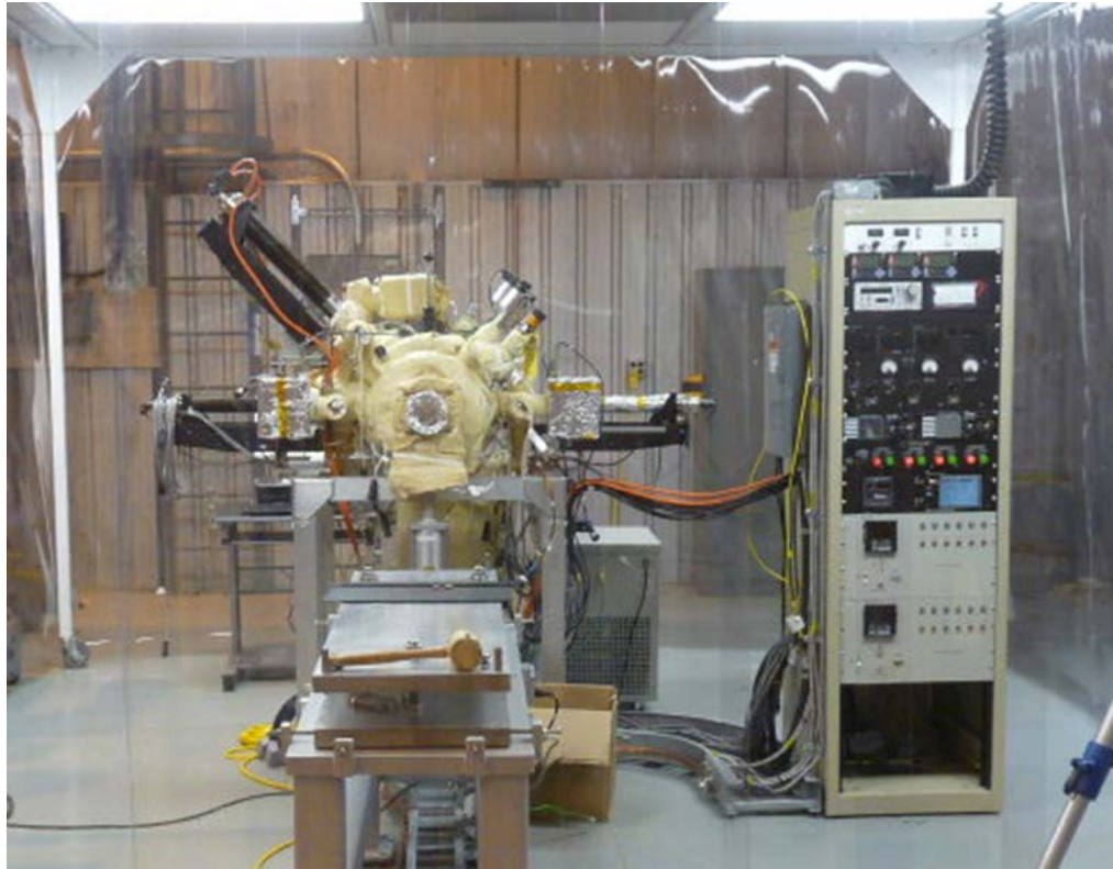
Figure 3-2. The photocathode deposition chamber. The “arms” seen projecting from the central vacuum chamber contain the alkaline sources.
