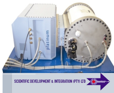
Figure 2-15. The commercial 10-atm CO 2 laser manufactured by SDI Ltd. (RSA).
