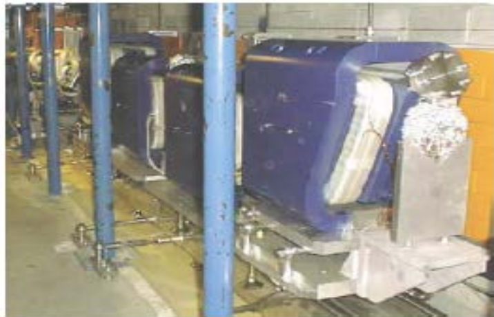
Figure 1-4c. The chicane compressor installed in the H-line.
