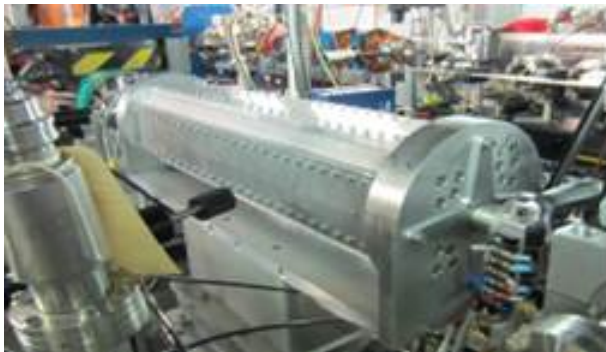
Figure 1-37. Picture of the RUBICON helical undulator installed into the ATF's beam line.
