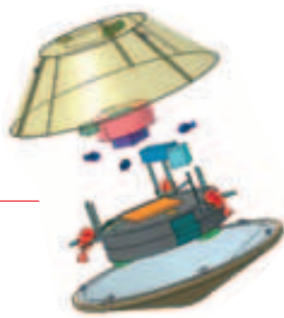
Figure 5.1.3.1: A possible design of a 50 kg lander for Mars with a payload mass of ~12 kg. The complete system including the EDLS would require about 150 kg for a secure landing. Two landers of this class could be accommodated on an orbiter like Mars Express, and inserted into a controlled manner from a highly elliptical Mars orbit. (ESTEC Concurrent Design Facility DemoLander study performed for the Exploration Programme/General Studies Programme.)
