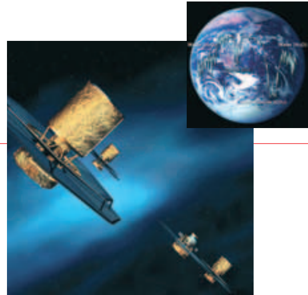
Figure 5.1.2.1: The near-IR nulling interferometer using a 4-spacecraft constellation at L2. The three beams collected by the telescope spacecraft are brought together on the central beam-combiner. A constellation of four appears to be the minimum required to establish the atmospheric characteristics of terrestrial planets (inset) within the habitable zones of stars within 25 pc.
