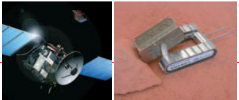
Figure 5.1.3.2: The release of one of two landers from a Mars orbiter before the initiation of the EDLS (left). On the surface, the lander would also require a mobile element (right). Here, a European mini-rover with a range of 50 m and carrying a geochemistry payload of 1 kg is shown.
