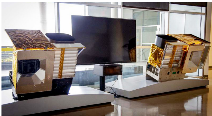
Models of the GOES-N Series imager (left) and sounder (right) instruments that are located in the lobby of NOAA's Satellite Operations Facility (NSOF) in Suitland, Maryland. Credit: NOAA
