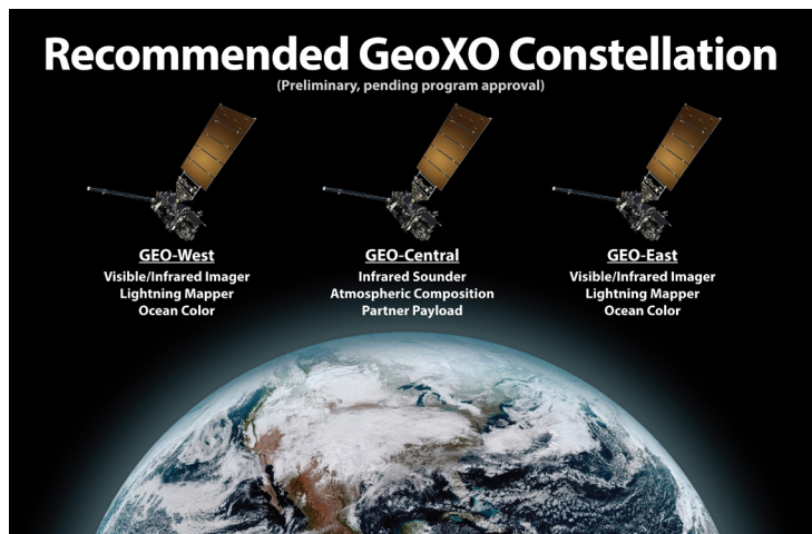
An ocean color instrument in geostationary orbit will provide observations of ocean biology, chemistry, and ecology to assess ocean productivity, ecosystem change, coast/inland water quality, and hazards like harmful algal blooms. Credit: NASA
