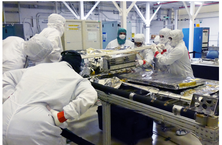
GOES-U SUVI telescope and electronics box installation. Credit: Lockheed Martin
