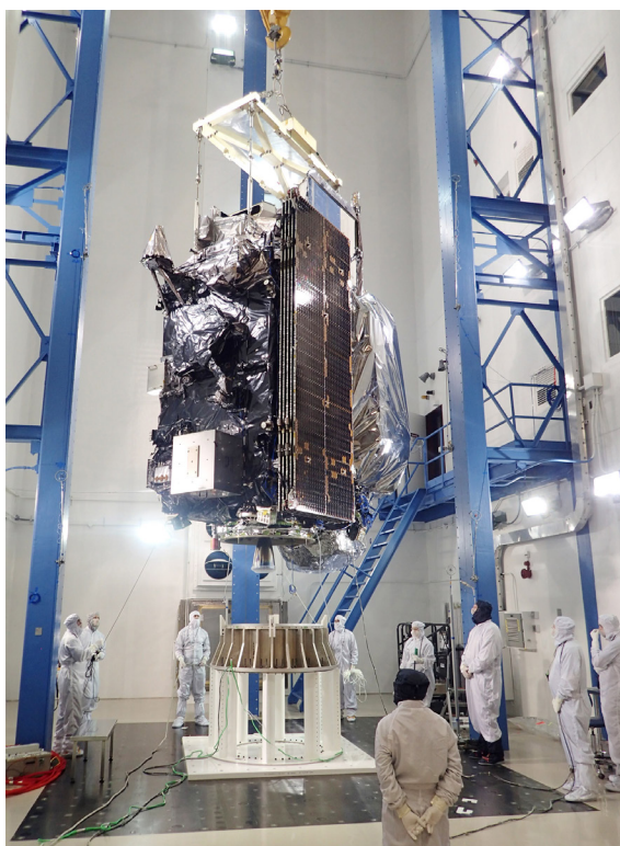
GOES-R acoustics testing. Credit: Lockheed Martin
