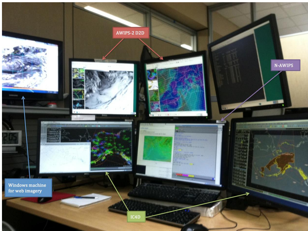
Figure 5. AAWU operational workstation containing IC4D, AWIPS-2 D2D, and N-AWIPS screens along with one Windows monitor for web displays
