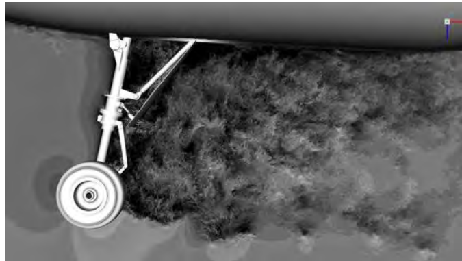
Figure 12: Simulation using Intel CPU version of LAVA Lattice Boltzmann of nose landing gear, where colors indicate velocity magnitude (white is fast, black is slow)
