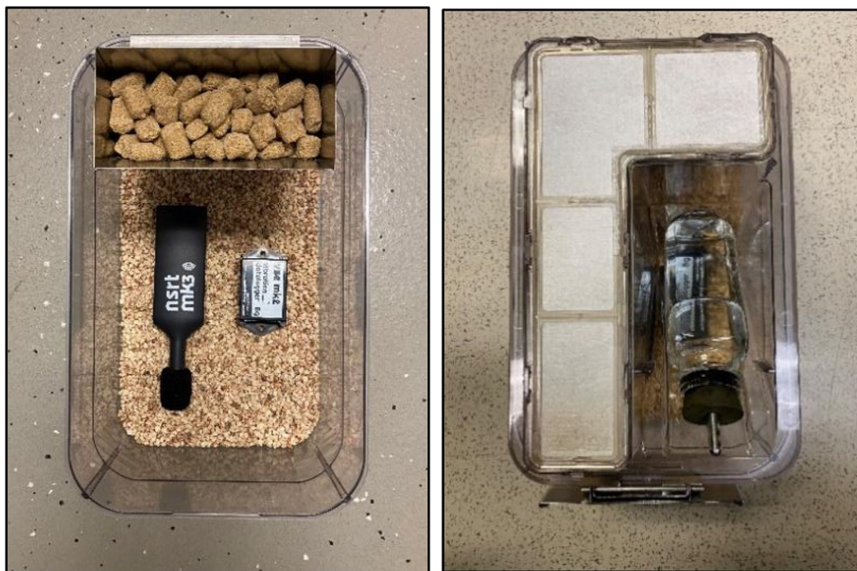
Figure 1. Setup of sound and vibration meter cage. Left: cage interior: sound meter placed on left on cage floor, vibration meter placed on right of cage floor. Right: cage exterior.
