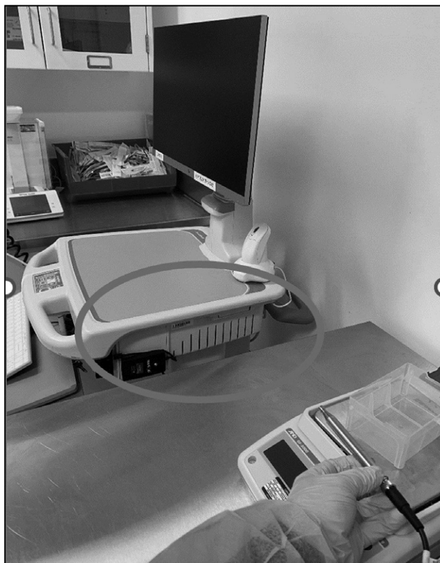
Figure 2. Computer generating USN near animals in a research lab. The oval outline indicates the source of USN from the cart-mounted computer. A clear acrylic or other solid barrier between the computer and weighing station would prevent the transmission of USN to the animal.
