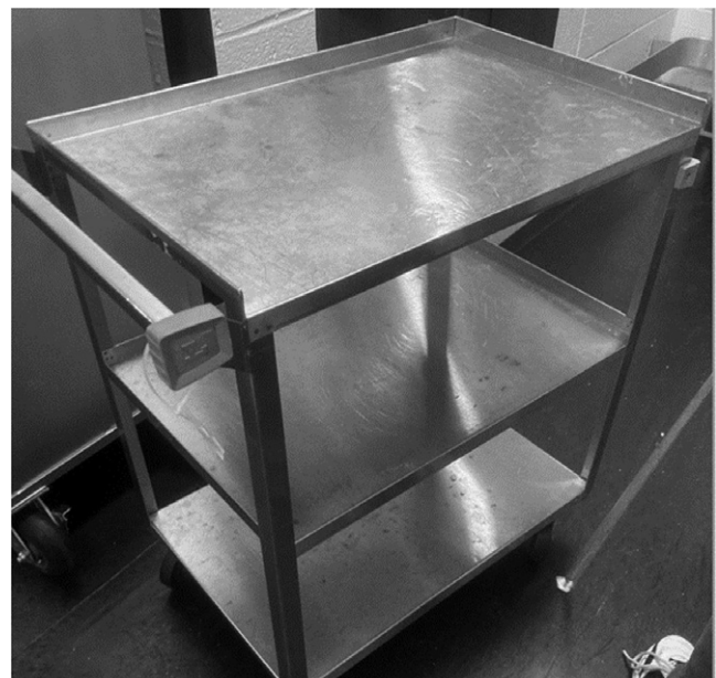
Figure 3. Typical light-gauge stainless steel animal facility transport cart, which can generate excessively high levels of noise and vibration for animals transported in cages.
