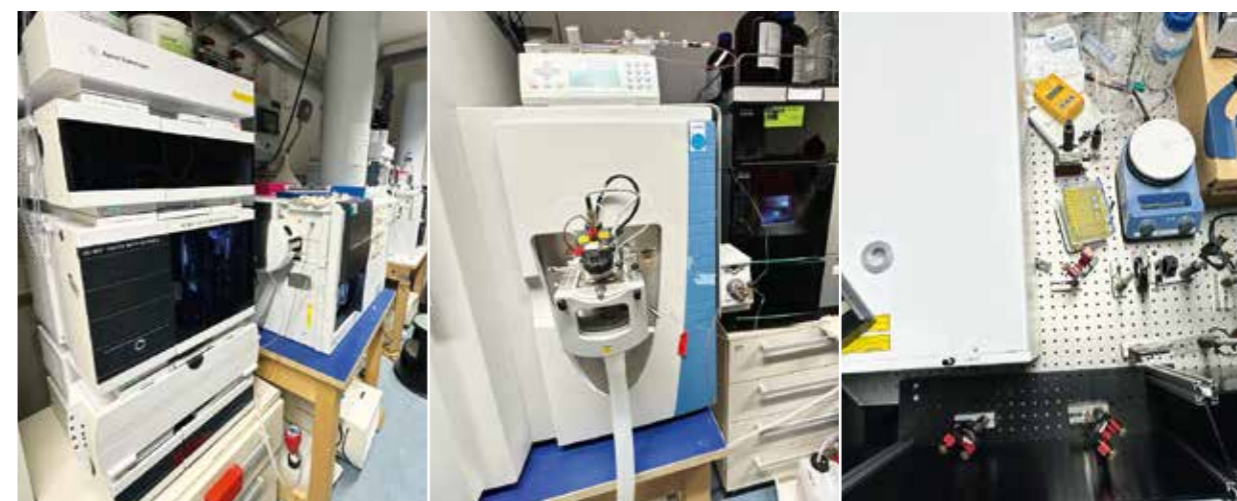
Instruments of the ORIGINS Ice, Dust and Sequencing Lab showing a high-resolution HPLC-ESI-TOF mass spectrometer, a HPLC-Orbitrap mass spectrometer and a DPSS UV-laser. The lab equipment is open to origin of life researchers in Munich and serves as a hub for manipulating and probing prebiotic molecules. It is located in downtown Physics at the LMU in the AG Braun. © AG Braun
