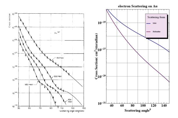
Figure 2: Elastic scattering data on Au at 84 MeV (upper curve) from Ref. [1](left) compared with this calculation (right). Also shown in the upper curves of this calculation are the cross sections obtained without form factor suppression.
