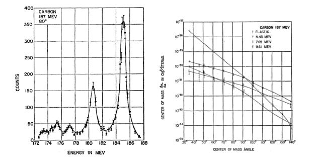
Figure 4: The left panel shows the energy spectrum seen at one angle ( $80^0$ ). This spectrum results from energy loss due to nuclear excitation since  $E_{scattered} = E_{beam} - E_{excitation}$ . The right panel shows the angular dependence of the elastic and inelastic rates.
