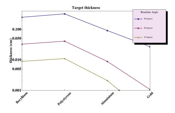
Figure 1: Calculated thickness (in centimeters) of scattering foils needed to produce 0.5 scattered electron/pulse in an aperture of  $1^0$  or  $10^{-3}$  steradians.
