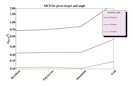
Figure 3: Multiple Coulomb scattering in the forward beam due to different choices of foil thickness.
