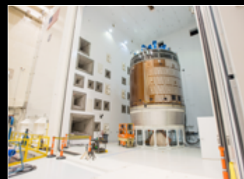
Acoustic testing, Structural Model
