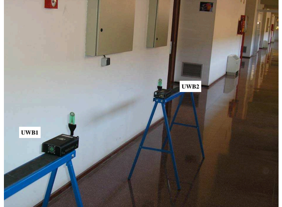
Fig. 3. Scenario considered for UWB range characterization in LOS. Experiments have been conducted in this 3 meters-wide corridor, varying the distances between antennas from 1 to 10 m.
