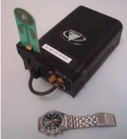
Fig. 2. A PulsOn transceiver. Four of these devices have been employed for the experiments described in this article.
