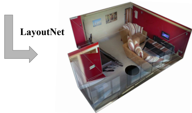
Figure 1. Illustration. Our LayoutNet predicts a non-cuboid room layout from a single panorama under equirectangular projection.
