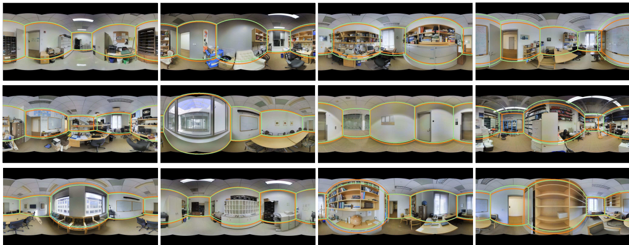
Figure 4. Qualitative results (randomly sampled) for cuboid layout prediction on the Stanford 2D-3D annotation dataset. This dataset is more challenging than the PanoContext dataset, due to a smaller vertical field of view and more occlusion. We show our method’s predicted layout (orange lines) compared with the ground truth layout (green lines). Best viewed in color.
