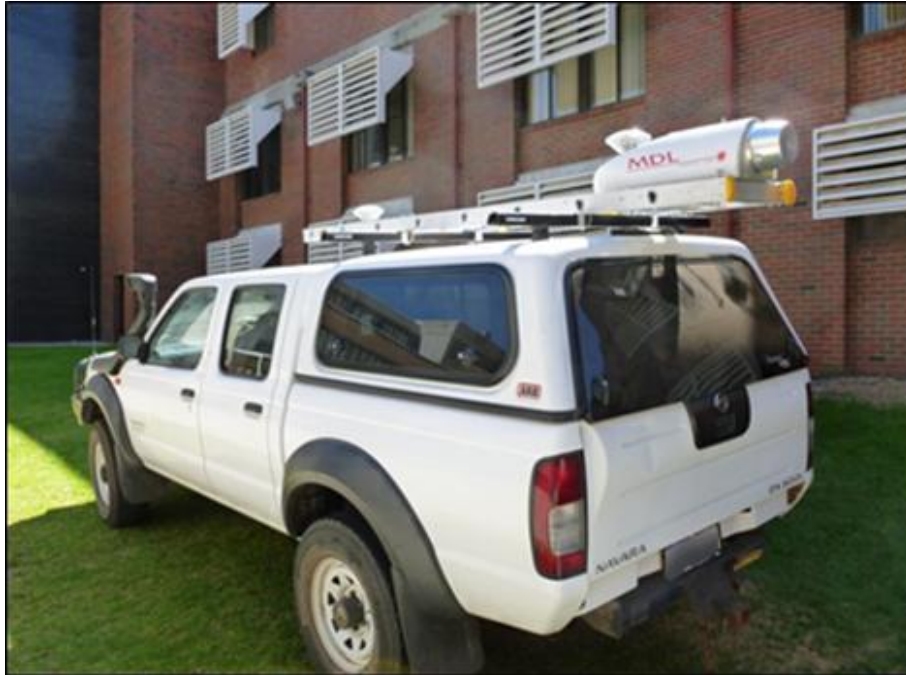
Figure 1: Mobile mapping vehicle with onboard sensors; (courtesy: Department of Spatial Sciences, Curtin University).
