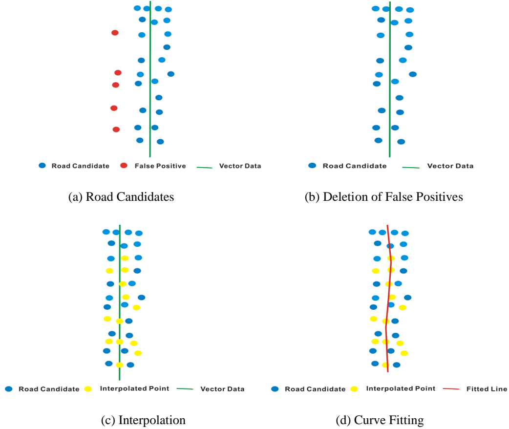
Figure 5. Refinement process: (a) road candidate; (b) deletion of false positives; (c) interpolation; (d) curve fitting
