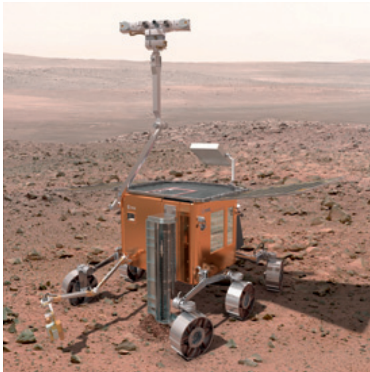
Figure 17: Artist's impression of the ExoMars Rover, which will search for traces of past and present signs of life by drilling into the Martian surface down to a depth of 2 m.
