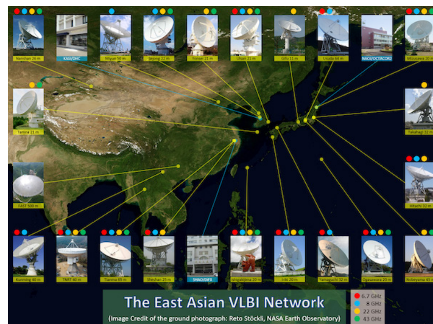
Figure 2. Concept map of the EAVN including the three correlator sites in China, Japan, and Korea. FAST 500 m telescope, which is to be used for EAVN observations at lower frequencies ( < 1.6 GHz), and the Thai National Radio Telescope (TNRT), which is under construction, are also included in the map. Photograph of each radio telescope and correlator site are overlaid on 'the Blue Marble' image. Credit of the ground image: NASA's Earth Observatory.
