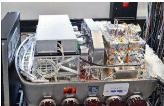
View of the GRAVITY instrument during construction. To the left of the image, the connections for the beam lines from the four VLT telescopes are visible. © MPE
