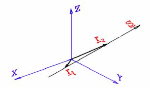
Fig 9. A line represented by two vectors
