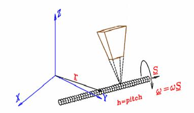
Fig 10. Instantaneous motion about a screw
