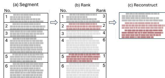
Figure 1: VDoc architecture. First, a long document is segmented (a), then each segment is ranked by its relevance to the question (b), and finally a virtual document is reconstructed with the top-ranked segments (c).
