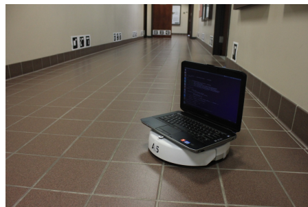
Fig. 16. A picture of the robot (an iRobot Create) operating in the office environment. Landmarks can be seen on the walls.
