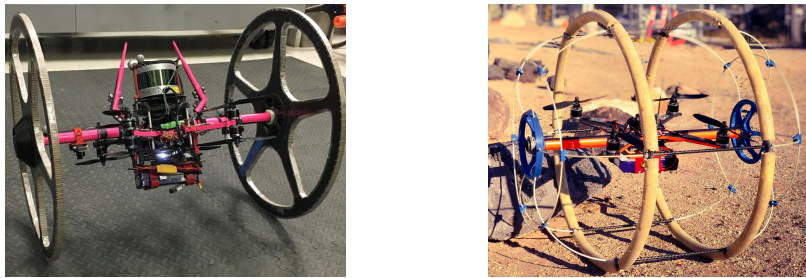
Fig. 2: Rollocopter platform (left) and Hytaq quadrotor (right). Our framework is applicable to any flying vehicle which can cope with collisions at moderate speeds.
