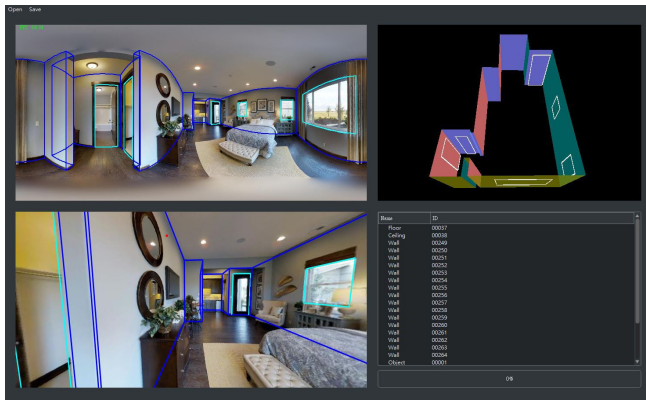
Fig. 4 We use PanoAnnotator [40] to annotate our MatterportLayout dataset. This figure illustrates the interface of the tool with PanoView (top-left), ResultView (top-right), MonoView (bottom-left) and ListView (bottom-right).
