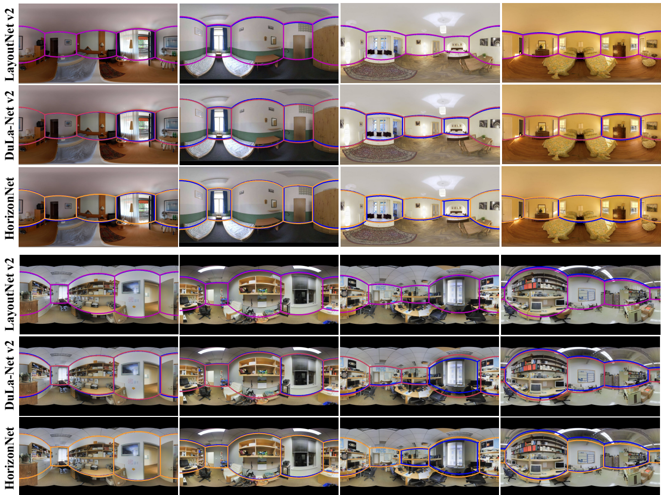
Fig. 10 Qualitative comparison on cuboid layout estimation. We show results selected randomly from the experiment of testing LayoutNet v2, DuLa-Net v2 and HorizonNet on PanoContext dataset (top) and Stanford 2D-3D dataset (bottom). In each example, we show the predicted layout (LayoutNet v2: purple, DuLa-Net v2: red, HorizonNet: orange) and the ground truth (blue) under equirectangular view.
