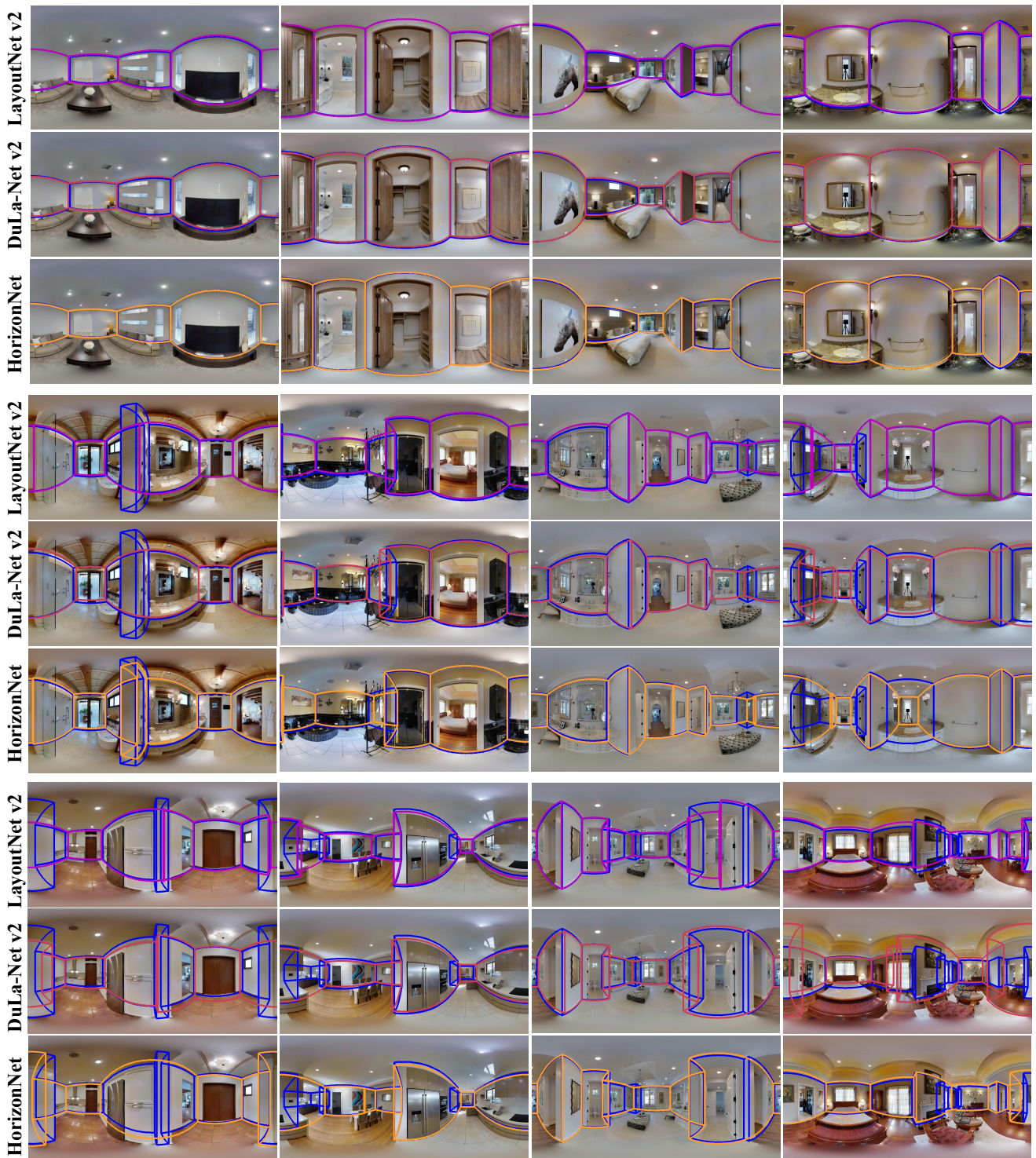
Fig. 11 Qualitative comparison on the MatterportLayout dataset. We show the 3D room layouts with various complexities estimated by LayoutNet v2, DuLa-Net v2 and HorizonNet. In each example, we show the predicted layout (LayoutNet v2: purple, DuLa-Net v2: red, HorizonNet: orange) and the ground truth (blue) under equirectangular view.
