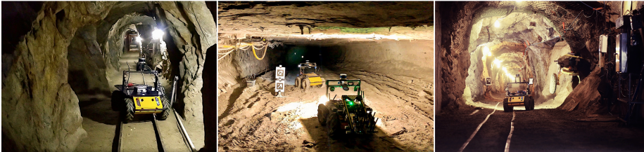
Fig. 16 Examples of the sensor-degraded underground environments explored by autonomous ground robots (Husky A200). From left to right, Eagle Mine in Julian, CA, Arch Pocahontas Mine in Beckley, WV and Edgar Mine in Idaho Springs, CO.
