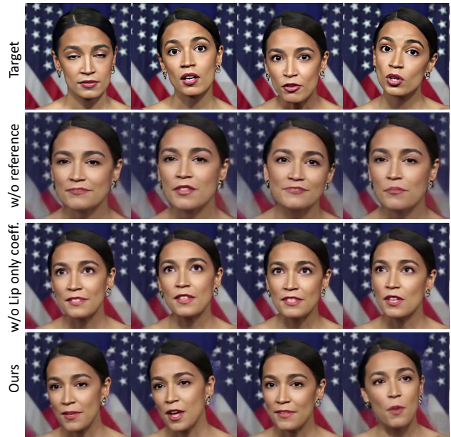
Figure 8. The ablation of ExpNet. We choose four frames from the generated video as comparison. Our method largely reduces the uncertainty of audio to expression generation. The reference \beta_0 is used to provide the identity information while the lip only coefficients generate better lip synchronization. Notice that, the target image is provided as the identity and lip motion reference.
