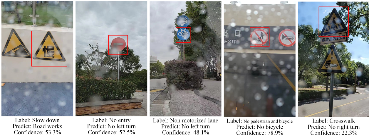
Figure 5. Adversarial raindrop examples captured in the real-world and the corresponding classification results.
