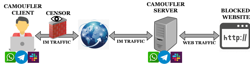
Figure 1: Camoufler basic architecture.
